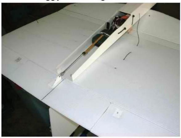
Set CG by placement of radio gear. For a very stable airplane, set CG on forward airfoil fold. For better slow flight response we have gone as far aft as halfway between folds, but high speed pitch response becomes very sensitive. Make your control surface throws barn doors! I went as far as I structurally could using standard sized servo arms.
